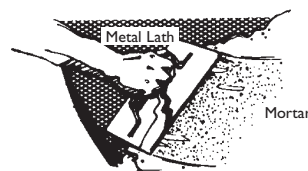
Figure 6 Apply mortar using a plasterer's trowel.
