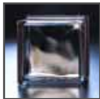
SRT™ Block, Clear and Wavy Patterns — Brown Edge Features a metal oxide coating on the inside surface of the block which greatly reflects solar energy while reducing the passage of sunlight.
